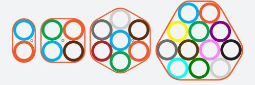
Höhle microducts are designed for long term protection of fiber optical cables. Direct Bury (DB) type of microducts are thick wall products that attain their mechanical robustness and functional performance through their intrinsic thick walls and need no further protection at underground installations. Höhle microducts conform to BS FN 61386 and BS FN 60794-5.
